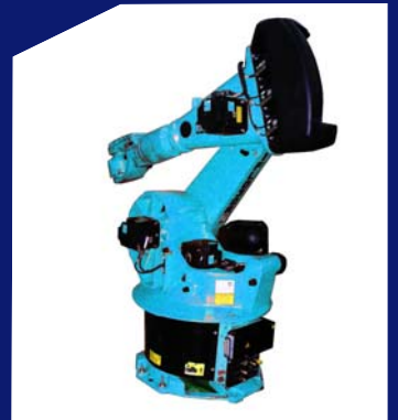
Scan Head with Remote Electronics in Robotic Welding Application
